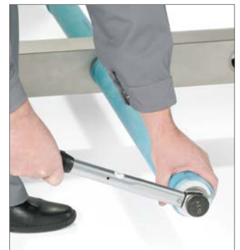
Fig. 5: Fitting with torque wrench
